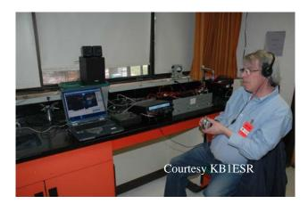
Above is the secondary station with tracking computer, rotator control, radio, and power amplifier. Joel W1JMM and Les N1SV operated this station. Based on a paper table of time vs. azimuth bearing Les and Joel kept the 14 element yagi aimed at the ISS should we need to switch. Since this antenna was ground mounted its horizon was higher than the tower mounted 22 element antenna. This would have resulted in a shorter available pass time if we had had to switch to it.
