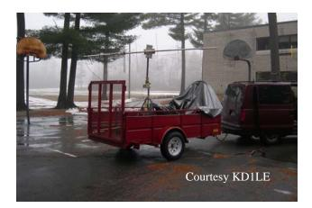
The backup antennas arrived ready for deployment. The secondary yagi was transported assembled with its coax and rotator cable rolled and attached to the tripod. The base for the yagi was on wheels so it could be quickly rolled into the field. The vertical used a tripod base and a ten foot mast and was assembled on site.
