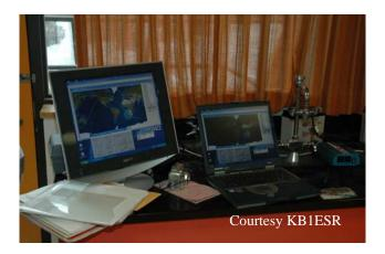
On the left side of the primary station was the tracking computer with software to track the space station and the controller interface software to pass tracking information to the controller interface.
