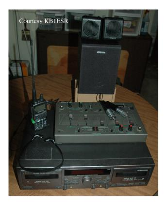
The connections are as follows. Microphone 1 and 2 to the respective inputs of the mixer board, secure the # 1 microphone to the microphone used to drive the transmitter (uplink audio). The # 2 microphone is pointed in the direction of the receiver speaker as a backup to the direct connection between the receiver and the mixer board (downlink audio).
