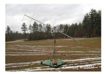
Above is the backup cross polarized antenna with an azimuth only rotator. The antenna was set at a fixed elevation. The antenna system was mounted on a wheeled base. Cables were kept connected to the antenna and rotator and coiled on the cart ready for quick deployment. This setup required an operator to monitor the time and manually make azimuth adjustments.
