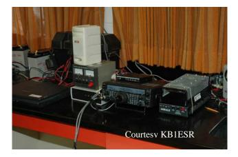
Above is the primary station with the packet computer on left (closed), rotator control and interface under the speaker and the radio with packet TNC on top. The power amplifier is on the right with the screen cover supporting two cooling fans. Stan KD1LE operated this station.
