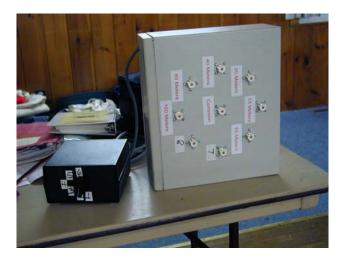
Stan KD1LE showed the eight port antenna switch he built for switching HF antennas at Field Day.
