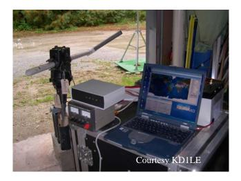
Below is a picture of the antennas we will use. On the left is a circularly polarized 22 element antenna and in the front center is a 14 element antenna.
