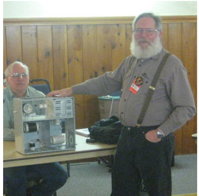
Bob W1XP displays the 600 Meter Low Pass Filter he designed and built. Looks like the Big Brother to the Ugly Field Day Filters. Instead of using a PC
