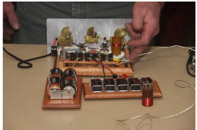
Leo K1LK showed a regenerative receiver he built based on early 1910's design.
