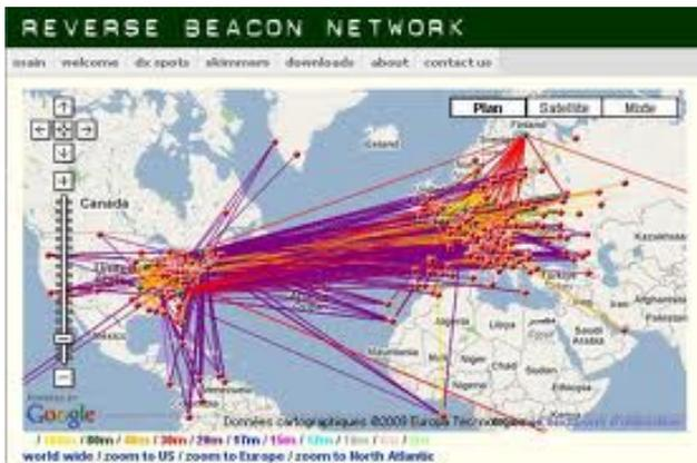
Another trend in the last several years is the Reverse Beacon Network (RBN). Stations with an SDR and an antenna can monitor a portion of a band and report the stations they hear on CW along with their associated signal strengths to a central server. This allows the reverse beacon network to provide a real-time indication of band openings. I have participated in RBN using my SDR-IR from time to time. For more information on the RBN pro-
