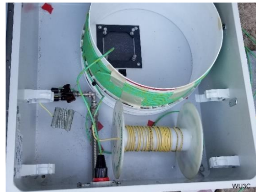
The matching network at the base of the antenna.
