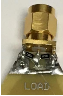
Figure-2, Installation of the two resistors
