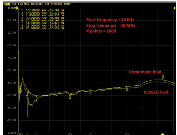
Figure-4A, Homemade load Vs 85052D load (10 KHz – 30 MHz)
