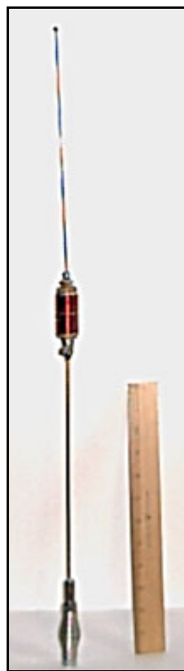
The 10-meter airmobile contest antenna.
