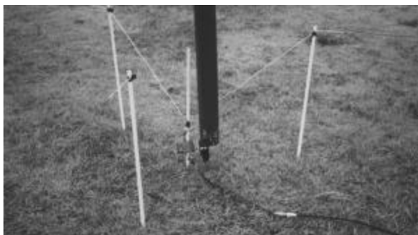
Figure 3, Base of Raised Radial Vertical Antenna. Note the bottle insulator, coil and relay box. See text.
