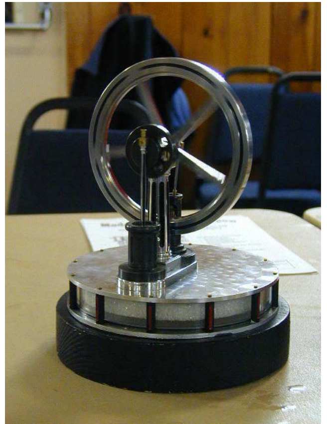
Demonstration Sterling engine which ran on a difference in temperature. During the meeting it ran on snow which was placed in the base. This was a cooler than the room temperature plate on top. Later it was run from the heat from being held in two hands which were warmer than the room.
