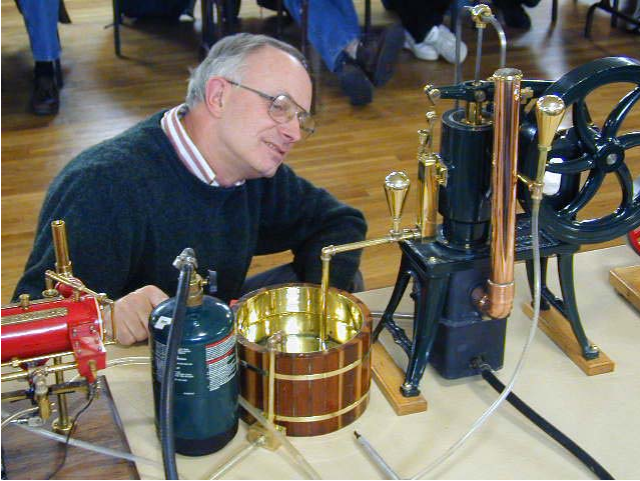
Above Norm is tending to a Sterling Engine which runs a water pump to supply cooling water to the double acting cylinder engine on the left and below.
