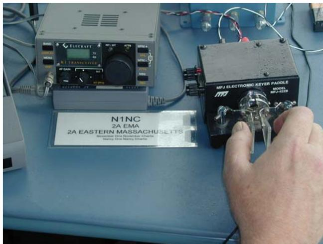
The CW station used Wolf's Elecraft K1 QRP transceiver that is on the left. On the right is an MFJ keyer and behind that is a three channel head-phone amplifier so multiple people use headphones and can adjust their sound level independently. We also used Bob's Ten Tec Scout to cover several other bands.
