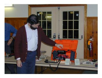
Ralph KD1SM, ARES box with two mobile rigs and batteries for rapid deployment, Powerpole distribution box with recessed connectors and individual circuit fuses
