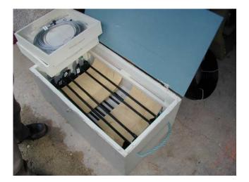
Above is the case containing the temporary guy wires and screw anchors that are part of the kit which makes setting up anywhere a possibility.
