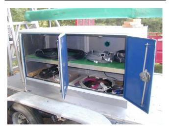
The tower trailer is loaded with all the antennas and cabling for the CW station. It also has the slings and other attachment equipment to protect trees or other objects that can be used as temporary anchor points.
