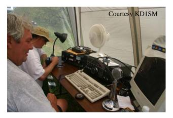
Above Peter N1ZRG and Les N1SV operate the SSB station. The two six port switches on the tuner (center top) were to select the antennas and filters. Whoever thought to bring the fans was a genius.
