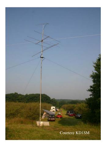
Above (top – bottom) are the antennas for satellite, six meters, and two meters
