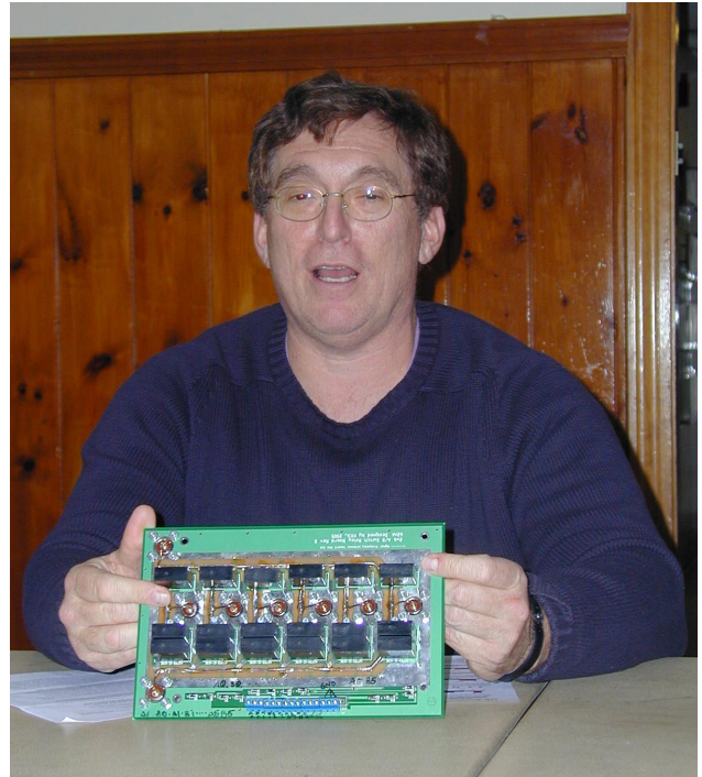
Bruce K1BG showed a two to six port antenna switch. The top picture shows the relay side of the board and below is the connector side.
