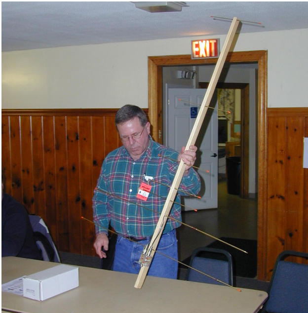
Leo K1LK showed the two meter and 440 MHz satellite antenna built.
