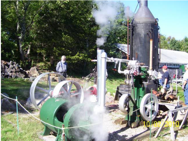
Bob W1XP looking over a steam turbine and generator (foreground left) and a steam engine (right) powered from the wood fired boiler (right rear).
