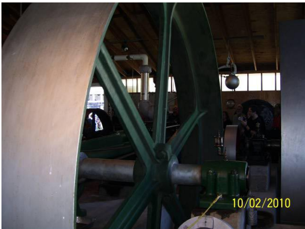
There were many engines housed inside. The above engine had a flywheel about 12 feet in diameter and had a piston bore about 36 inches. It was operating most of the time we were there.
