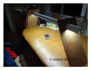
With a \$5 LED shop light for the illumination I used two pieces of Masonite as supports. I used a holesaw to cut a three inch hole in each for the light to slip through. If the support is sufficiently wide the light is quite stable.
