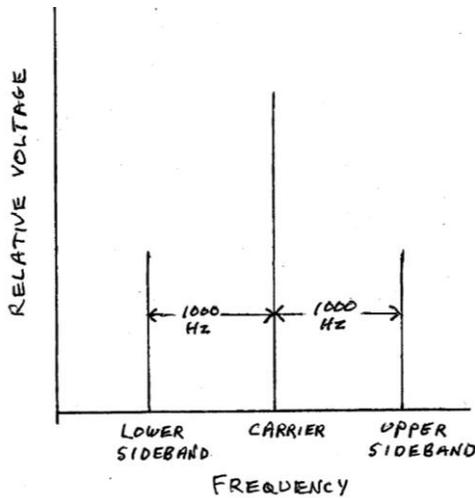
modulation of a carrier by a single 1000 Hz tone, in the frequency domain.
