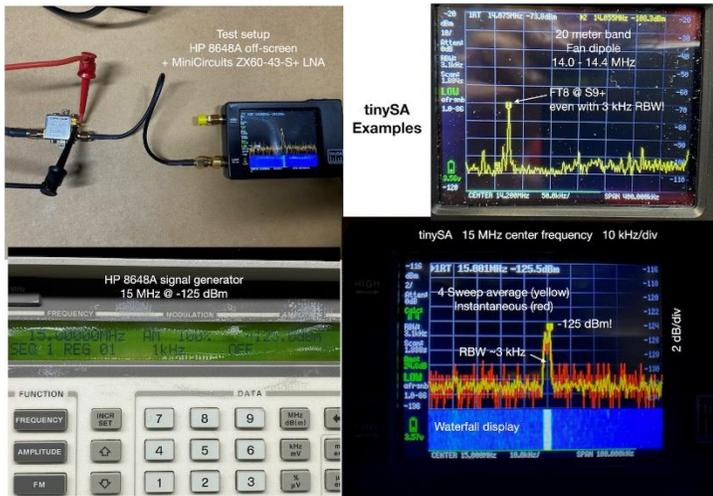
John, AE5X, has demonstrated another skill example using the tinySA as an approximately calibrated signal generator with a handful of external attenuators to do a MDS measurement on a receiver. The result comes within 1 dB of published specs – see:
