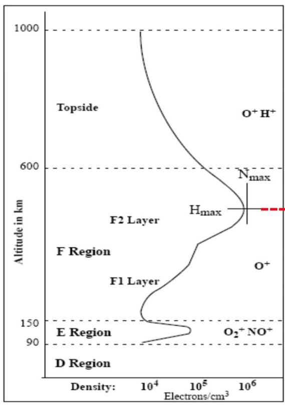
Example daytime ionosphere electron density profile. Shape changes and/or overall increases in electron density can cause effective propagation path length changes, producing apparent frequency shifts.
