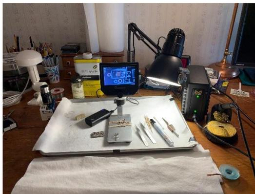
I had been using a jeweler's "OptiVisor" magnifying visor, and a Hakko soldering rig, but I was constantly having to adjust the visor, and lean way over the work. Also, I found that I had to set the solder tip temperature significantly above the SMD's recommended soldering temperature to get the solder to flow before my shaky hand would move the part out of alignment.
