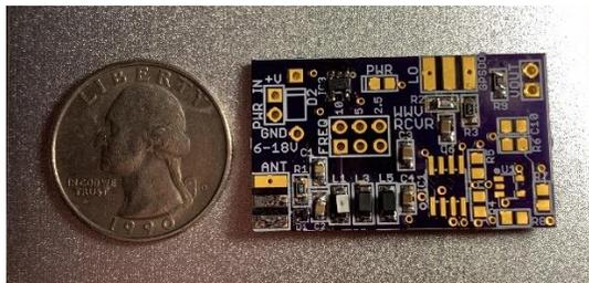
I set up a solder station in a white-felt-lined cookie sheet (white so I could see parts that jump out of my tweezers, and felt so they would be less likely to bounce). Even so, I managed to launch several SMDs into orbit, never to be seen again. Good thing I had ordered multiples of each!
