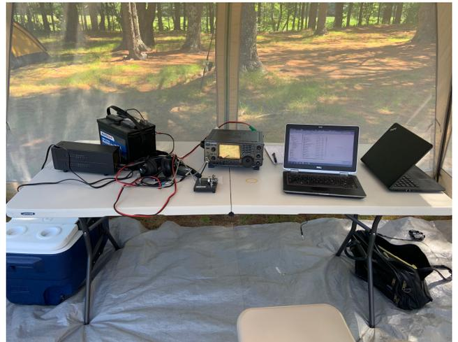
This year, I headed up on Friday morning and set up my station – consisting of an ICOM IC-746Pro and a 40 meter inverted V, situated in one of the screen rooms I bring on Field Day. The 746 ran off battery power, and I turned it down to 5 watts or so in order to conserve battery life. Conditions weren't the best, but on 5 watts rag chewed with people around the country and Europe on 40 meter CW. And I made a few contacts in the contest as well.
