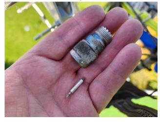
and minor repairs on the antennae feeders of N1MX repeater last month. They replaced a broken N to SO239 adapter and drained and
