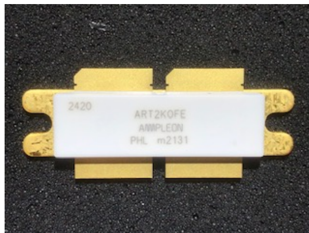
FIG 2. LDMOS ART2KOFE. It hosts two matched transistors. Good from HF to 0.4GHz.
