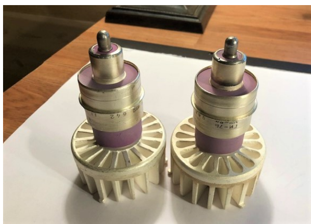
FIG 1. A pair of metal-ceramic VHF triodes 6L7B. These work at HF frequencies as well.
