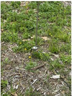
quarter wave at 14.08 MHz, the FT-4 frequency for 20 meters. I screwed the antenna into the base and added a 1:1 choke on the radio end of the feed line.
