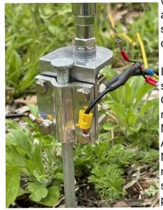
wires are attached to the spade connectors.
