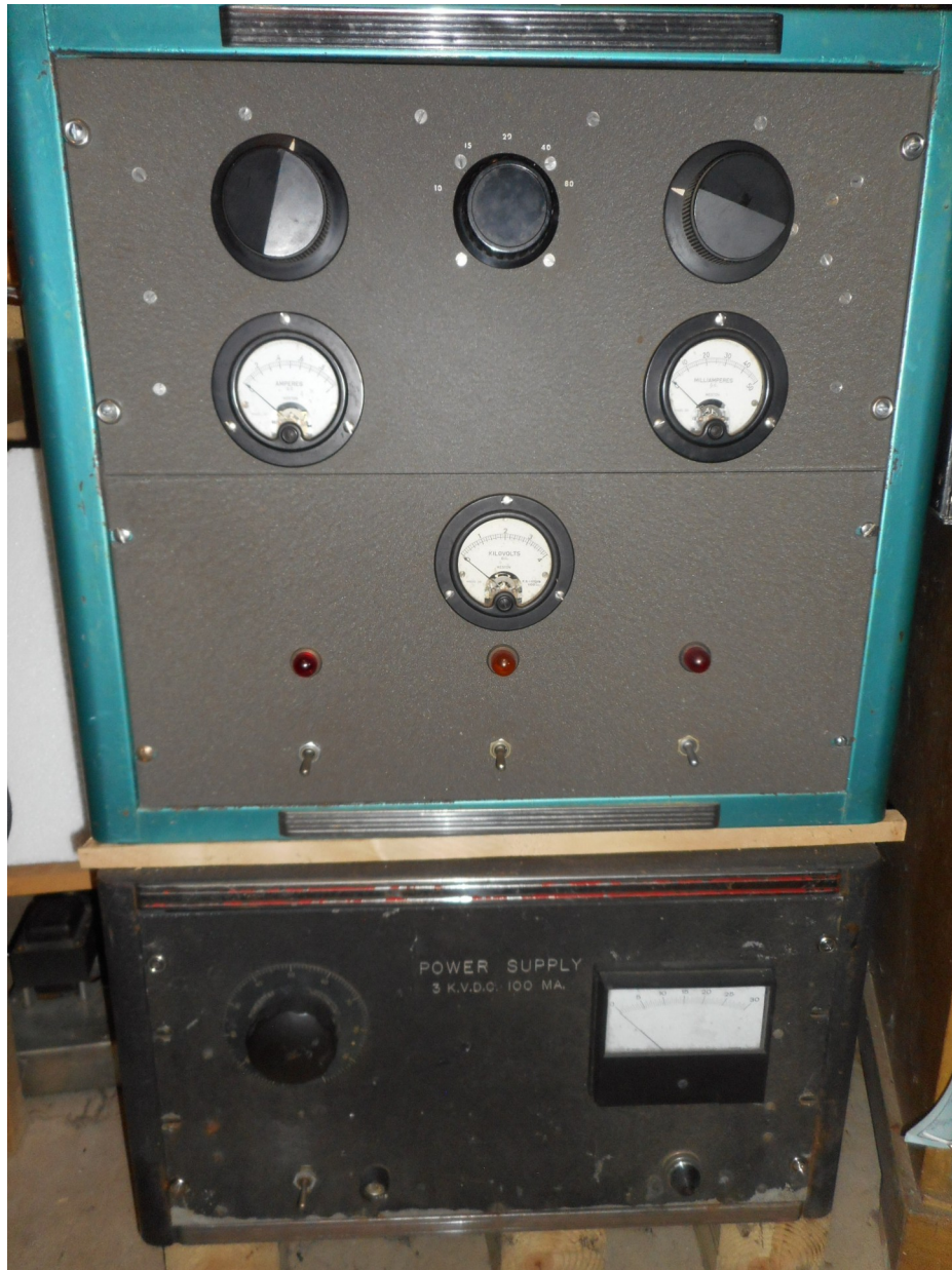
Figure 4 Amplifier and Power Supply Stack
