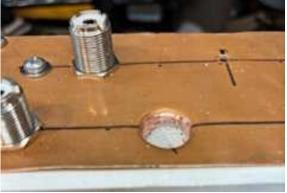
I replaced the copper, but lacking a proper 5/8" bit for metal, I used one of those step drills. As the copper is so soft, it was not so much drilled as swaged into the opening. I'd like to think this provides more contact area for the bulkhead connectors.
