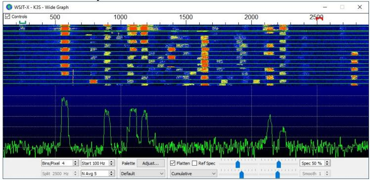
Both FT8 & FT4 are digital modes found in the WSJT-X software package. FT8 uses a 15 second T/R sequence. While FT4 uses a 7.5 second one. Below are the default FT8 & FT4 operating frequencies, however stations are free to define new frequencies within the WSJT-X settings Frequencies tab as needed. For further information on WSJT-X refer to the user's manual here
