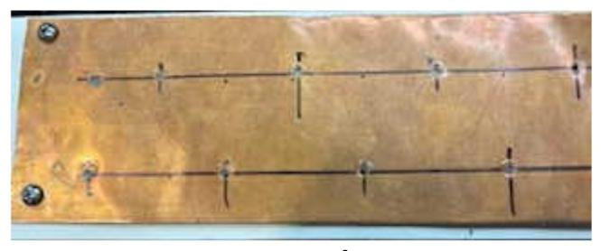
I removed the copper and drilled the PVC with a 5/8" spade bit. I learned quickly that PVC chips quite badly, so the remaining eleven holes were drilled from both side to minimize the chipping.
