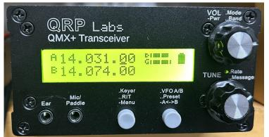
The QRP-LABS QMX+ transceiver is a 160 - 6m QRP transceiver that combines the single tone digital functionality found in the QDX transceiver with a basic CW transceiver. The QMX+ is larger than the QDX, but is still
