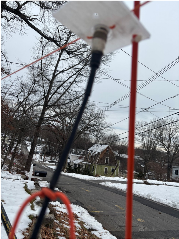
The feed point coax-side view showing the strain relief.
